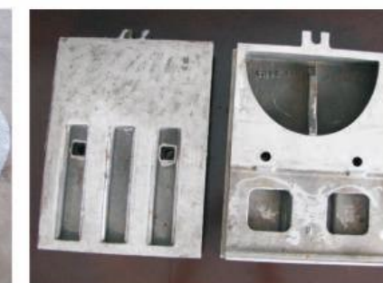
Cooler grate 篦板
